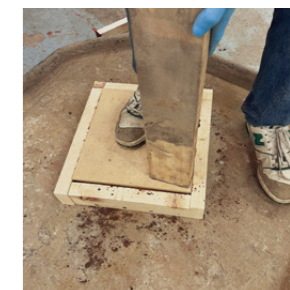
Process of mixing rammed earth mixture and compressing it into the CNC milled formwork
