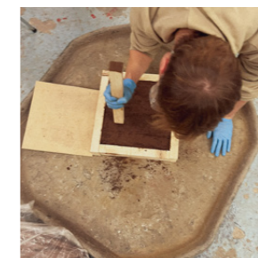
Process of mixing rammed earth mixture and compressing it into the CNC milled formwork
