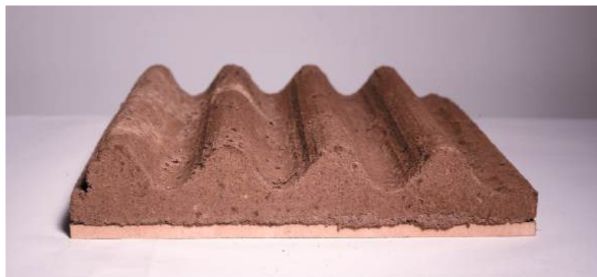
Dried results of the rammed earth panels made at 1:1
